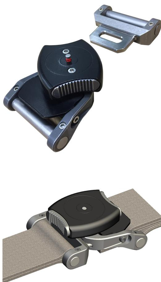
The Martin-Baker Rotary Emergency Aircrew Connector Harness (REACH) is designed for use with an ejection seat equipped with a Torso Harness restraint system. In order to optimise post-ejection aircrew survivability, REACH is ergonomically designed to provide simple operation in all environments, even with thick winter gloves.
