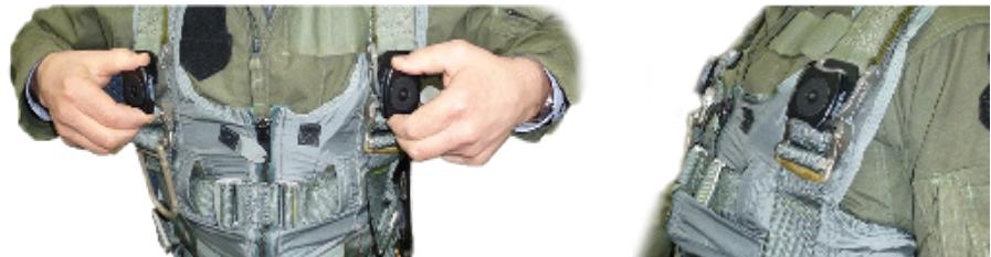
The physical and visual presence of the red indicator pin allows operators to establish whether the rotary release is in locked or unlocked release condition regardless of whether they can see it. Protrusion of the pin indicates a 'disconnected' state.
