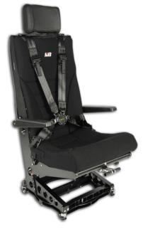
Since its certification and release into service in 2000, the Martin-Baker Rotating and Traversing Seat has been selected for applications including Police and EMS installations on the following platforms:
