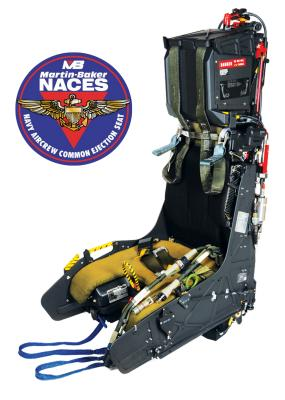
The US14A Ejection Seat is commonly known by the US Navy as NACES (Navy Aircrew Common Ejection Seat) from the program that originated it. The NACES Seat carries the US Navy designation SJU-17.
