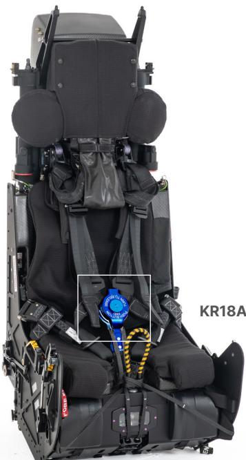
On initiation, the Quick Release Box (QRB) of the integrated harness is released by mechanical action of a small piston driven by a very small contained explosive charge.
